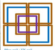
Blue coil : TX coil Brown coils : repeater array Purple coil : RX coil
